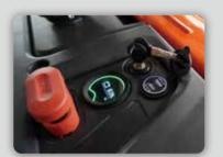
The multi-function instrument can display the vehicle working status, battery power, working time, driving speed and steering angle. When the vehicle fails, the outer ring aperture of the instrument will change from green to red, and the fault code will be displayed.
