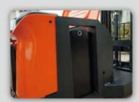
Standard side battery extraction, through a special trailer, battery replacement efficiency is high, the operator can operate the vehicle multiple shifts.
