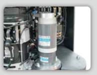
The standard electric power steering system used in other Noblelift stackers can quickly and accurately control the position of the steering wheel, while meeting the standards, with high reliability and safety.
