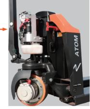
Easy Maintenance. Maintenance can be easily done just by removing the cover. And without removing the cover, you can only use the external programming port to diagnose faults.
