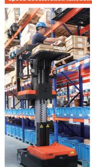
While platform is raising to its maximum height, the maximum available lift and drive speeds will go through three steps of speed settings according to the following lift height ranges for the platform: 0-500mm, 500-1500mm, 1500-3000mm to ensure the truck's stability and operator's safety.
