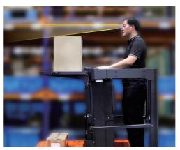
Adjustable height of the front shelf allows to ensure good visibility and avoid overlapping of operator's field of view by goods located on it.
