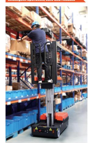
Both models are equipped with automatic closing doors preventing the operation of the truck when doors are opened.
