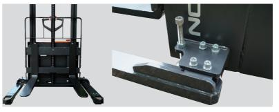
The support legs are fixed with screws located outside of the truck's body (4 screws for each side). The position can be easily adjusted according to the customer's needs to achieve the overall width of the truck: 46.5"/50.5"/54.5" 58.3".
